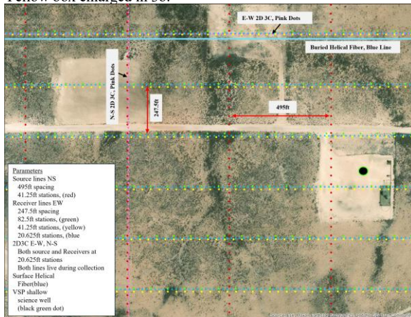
Figure 3b) Field test zoomed in showing 2D3C lines, VSP location, station spacings and line spacings of various equipment.
